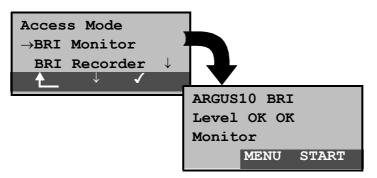
After starting the *Monitor* function, the ARGUS will first be in Monitor mode (the monitor is not yet active): the second line shows the evaluation of the level on the NT-side (first OK or << (too low), >> (too high), \_ (no level) and TE-side (second OK).
